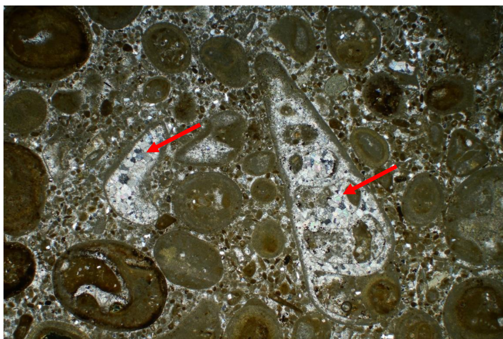
Figure 3. Sparite bioclasts (arrowed). Cross polarised light, magnification x25.
